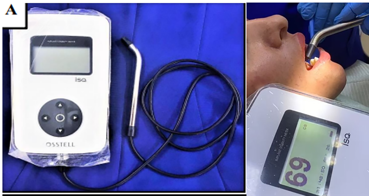
Figure 2: (Left) OSSTELL Stampgatan®, Sweden for Implant Stability Measurement, (Right) FRA Analysis for the Inserted Implant.
